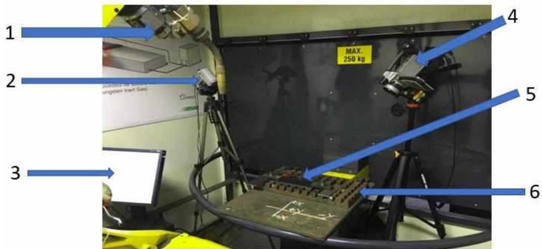
Fig 3.1 The robotic welding cell: 1. Fanuc 100 iB Industrial Robot 2. Raynger MX4 Infrared Pyrometer 3. PC for data acquisition from the pyrometer, 4. Infrared camera, 5. Base metal, 6. Modular fixture
