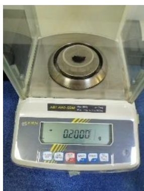
Figure 4.9. Weighing oxide nanomaterial Fe_3O_4 .
