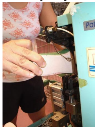
Figure 8.38 Attachment of the insole to the last
