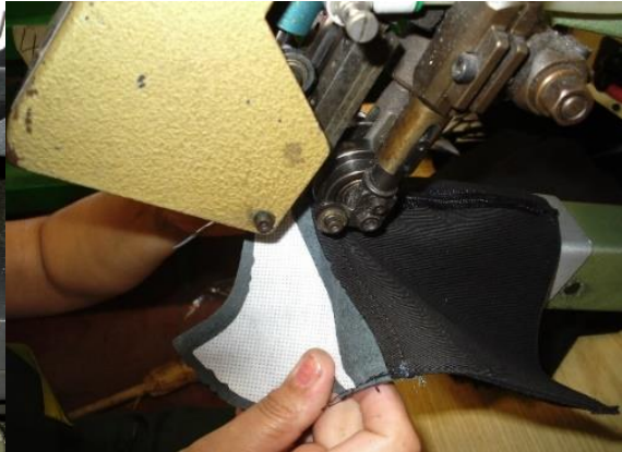
Figure 8.33 Smoothing machine and applied self-adhesive tape
