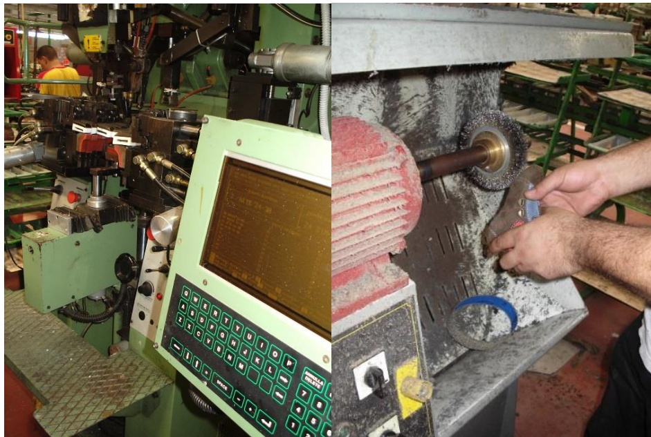
Figure 8.41 Rear pulling machine
