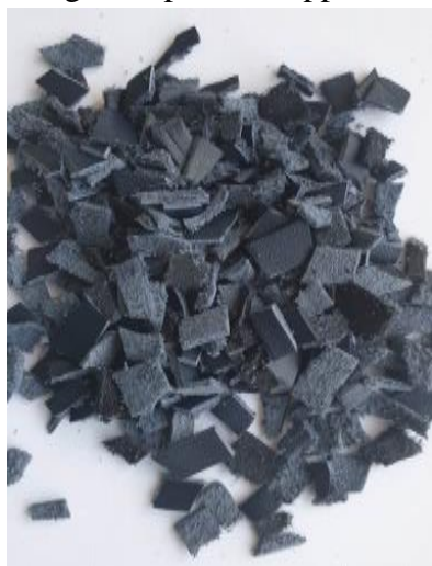
Figure 7.1 Ground protein wastes in a knife mill and sieve
