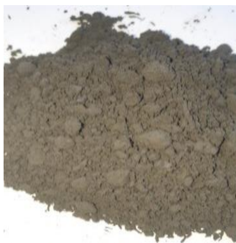
Figure 7.2 Ground protein wastes in a cryogenic mill
