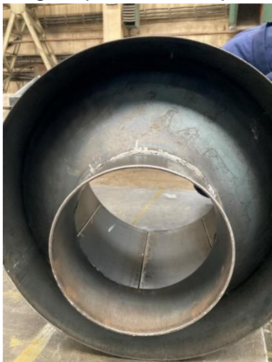
Figure 4.33. Manufacturing details inner cylinder with longitudinal slits
