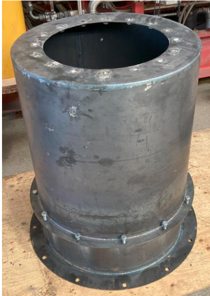
Figure 4.35. Manufacturing details outer cylinder filter separator
