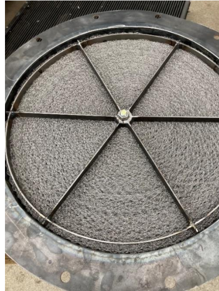
Figure 4.36. Manufacturing details demister T600- \phi 650x150 mm
