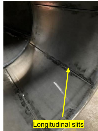
Figure 4.32. Manufacturing detail inner cylinder with longitudinal slits
