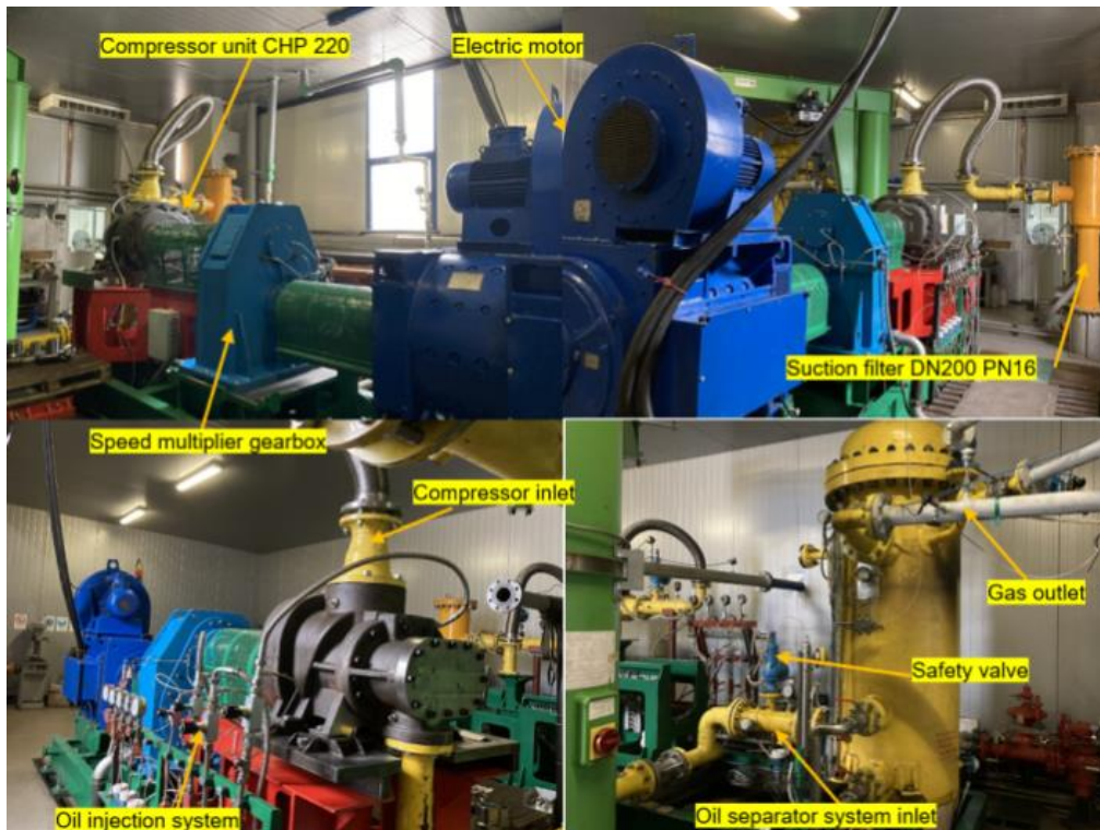
Figure 4.39. Experimental test bench.
