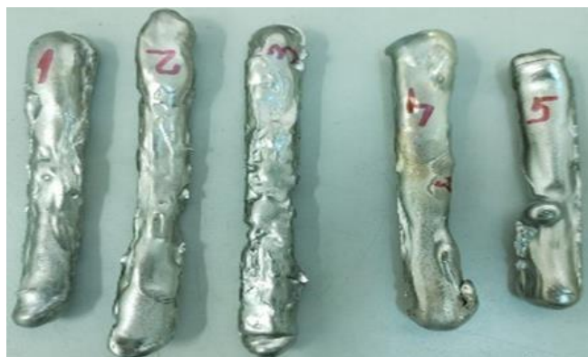
Fig. 4.2 Image of ingots obtained by melting RAV.
