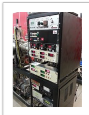
Figure 5.2. The command-and-control system of the deposition facility
