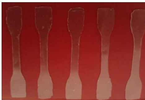
Figure 6.2 Test specimens of films made from hydrolyzed pectin for mechanical testing
