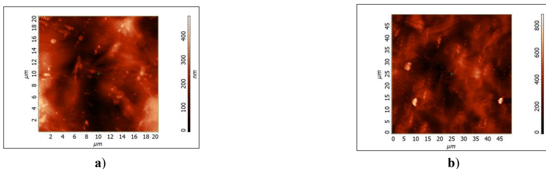
Figure 5.7 2D images of the AHO samples characterized by AFM: a) 20 × 20 μm; b) 50 × 50 μm
