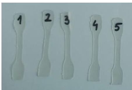
Figure 4.4. Specimens of corn starch-based films were prepared for mechanical testing
