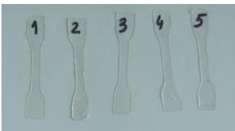
Figure 4.2. Specimens of potato starch-based films were prepared for mechanical testing
