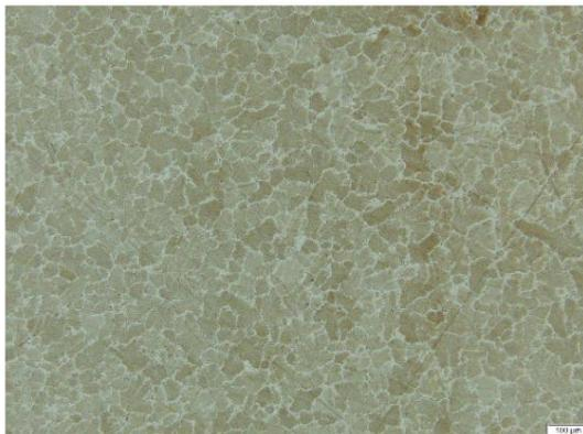
**Fig. 5.7.** Optical microscopy images of sample 5 – solution quality. Marble Attack ( $M = 100x$ );
