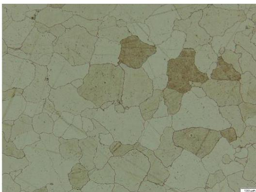
**Fig. 4.19.** Optical microscopy image of sample 1 – homogenized. Marble Attack ( $M = 100\times$  (a));
