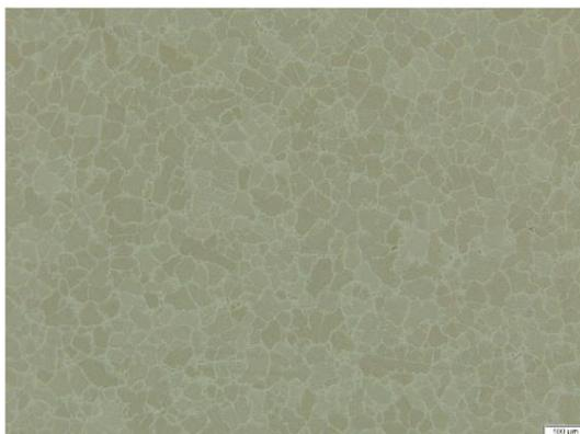
**Fig. 4.23.** Optical microscopy images of sample 5 – homogenized. Marble Attack ( $M = 100x$ ) (a);
