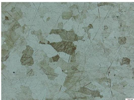
Fig. 5.3. Optical microscopy images of sample 1 – solution quality. Marble Attack ( $M = 100x$ );
