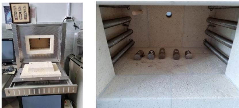
**Fig. 4.14.** Electric heat treatment furnace used for homogenization annealing
