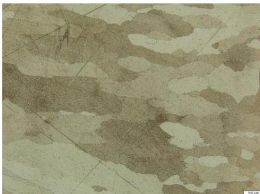
**Fig. 4.21.** Optical microscopy images of sample 3 – homogenized. Marble Attack ( $M = 100\times$  (a);
