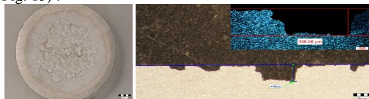
Fig. 12 - Appearance of macrostructural surfaces (left front section, parallel to eroded surface, right in cross section, background - optical microscope image, detail - stereomicroscope image) subjected to cavitation erosion of Al-Mg alloy, in cast condition, control sample.
