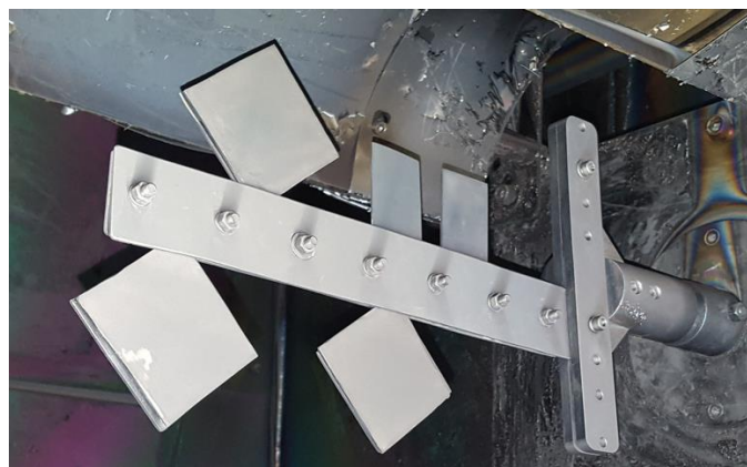
Fig. 6.4 EB- PVD deposition samples of (NiCrAlY)- ZrO 2 doped with CeO 2 -Al 2 O 3
