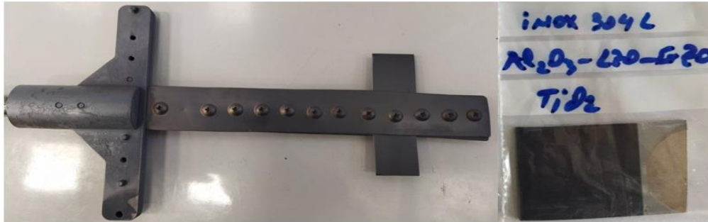
Fig. 8.7. EB- PVD deposition samples of (NiCrAlY)- Al 2 O 3 - LZO - GZO -TiO 2
