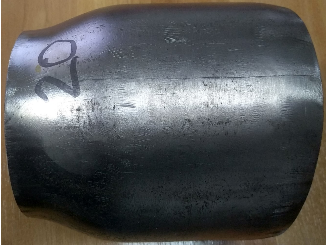
Fig. 38 - Plastic deformation of the pipe after use of the penetrator with the tip angle of 40°
