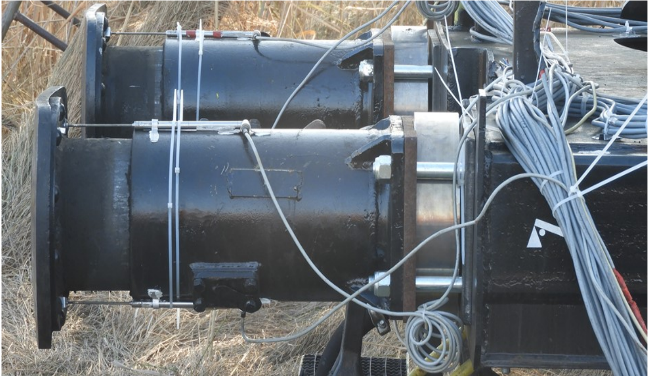
Fig. 33 - Mounting the sensor assembly on the two buffers
