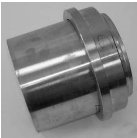
Fig. 16 - The device before plastic deformation of the pipe
