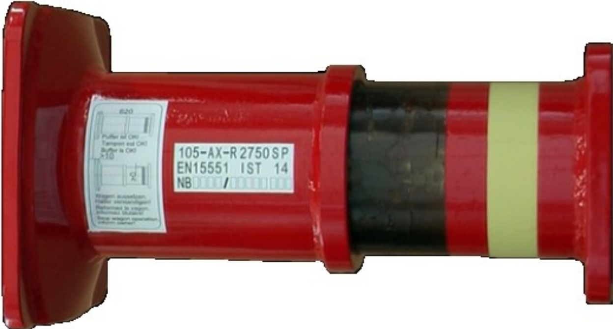
Fig. 1 - INNOVA buffer of 150 kJ
