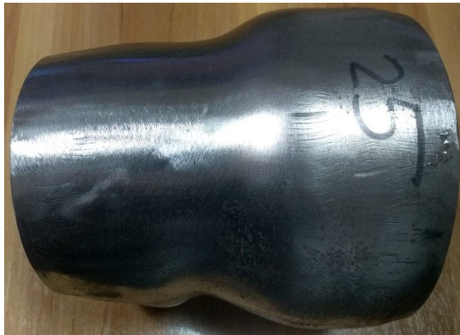
Fig. 39 - Plastic deformation of the pipe after use of the penetrator with the tip angle of 50^{\circ}
