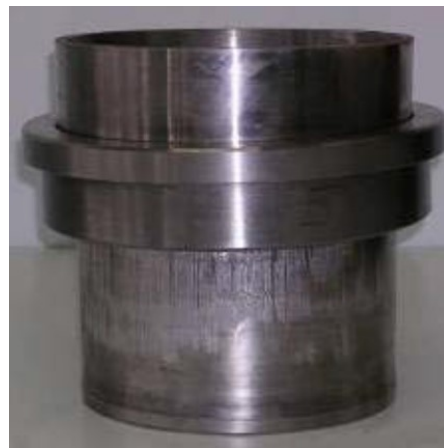
Fig. 17 - The device after plastic deformation of the pipe
