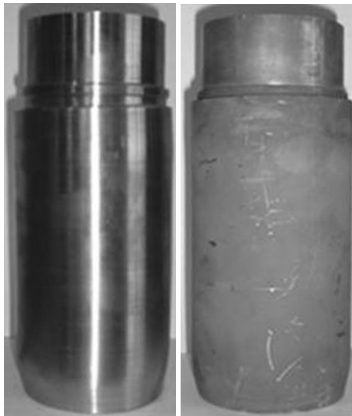
Fig. 14 - Pipe assembly after deformation
