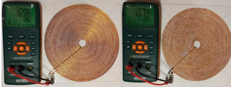
**Fig. 3.6.** Checking planar spiral coil self-inductance (coil type D, E)
