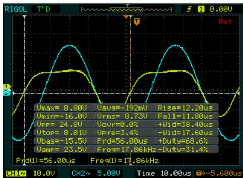
Fig. 1.4. Supply voltage waveform parameters for experiment 1
