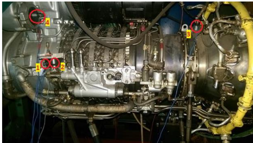
Fig. 12. Position of accelerometers on the TV2 turbine engine: (1) axial-horizontal near the harvester, (2) axial-vertical near the harvester, (3) at compressor end, (4) on the engine starter [100]
