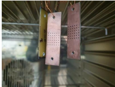
Fig. 6.5. Aged contact samples in the presence of sodium chloride (NaCl) solution in a forced-air oven.
