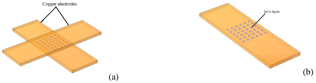
Fig. 3.8. Geometrical model (model IV) showing: (a) the copper electrodes, (b) the ZrCu spots at the interface.
