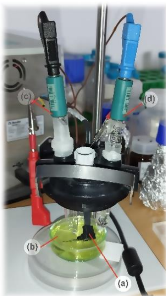
Fig. 5.2. Support for the 3-electrode cell: a) 3D-printed Working Electrode (WE); b) Redox solution; c) Auxiliary/Counter Electrode (CE); d) Reference Electrode (RE) [54] .
