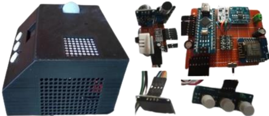
Fig. 3.36. The fully assembled ambient monitoring prototype device (left) and its internal circuitry (right)
