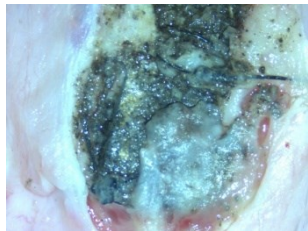
Figure 6.35. Appearance of the alloy sample from batch 1S Mg3Nd_A_CAHAp observed on the external face of Calvary after peeling off the skin (10x)
