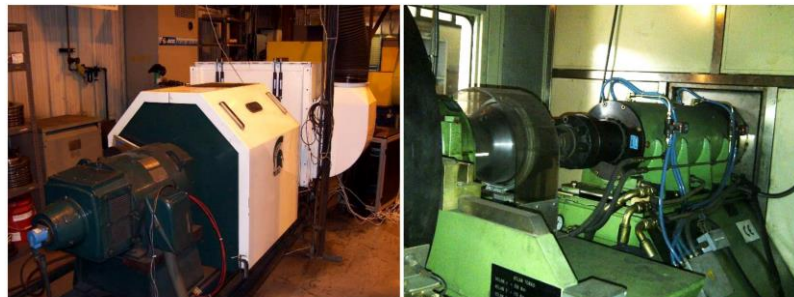
Fig. 4.5 Inertia dynamometers are used for tests [107]
