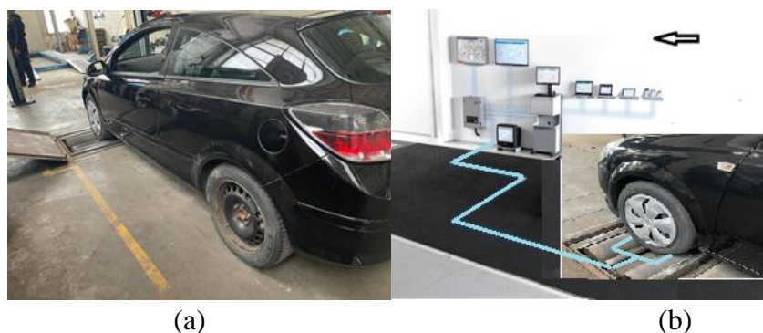
Fig. 5.10 Testing the front axle's brake system - Sample 1: (a) positioning the vehicle on the stand; (b) data collection method/signals and transmission to the database
