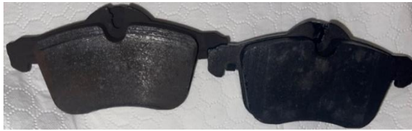
Fig. 6.1 Uneven wear of the brake pads on the front axle
