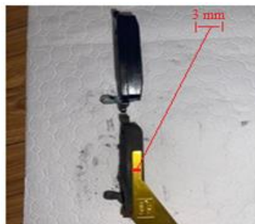
Fig. 6.5 The measurement of brake pad wear on the rear axle
