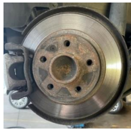
Fig. 6.4 Worn brake disc
