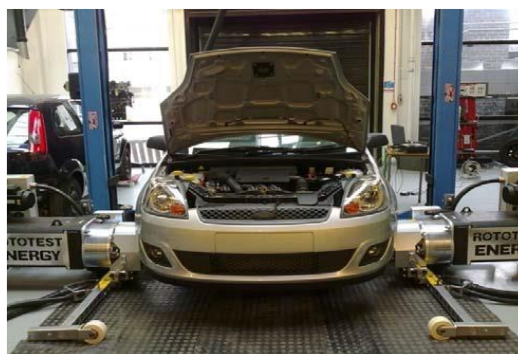
Fig. 4.3 The chassis dynamometer is attached to the front wheels of the car [84, 86] with the following specifications: maximum power output: 100 kW, which the vehicle can both generate and absorb; instantaneous maximum torque: 2500 Nm; continuous maximum torque: 1180 Nm; maximum hub speed: 2100 rpm, equivalent to the vehicle's maximum speed of 250 km/h.
