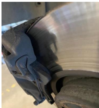
Fig. 5.5 Scratches and wear marks present on the surface of the brake disc
