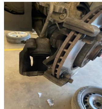
Fig 5.6 Brake disc with rust marks
