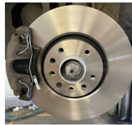
Fig. 6.5 New disc and pads assembly
