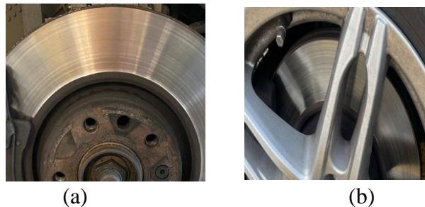
Fig. 6.12 The degree of wear on the brake discs: a) original brake disc b) aftermarket brake disc
