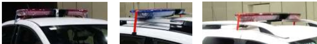
Figure 23 Location of light warning device
