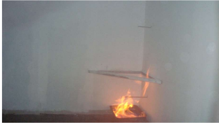
Fig. 20. Image after 30 seconds of pumping water into the enclosure at water temperature for suppression of 15 °C
