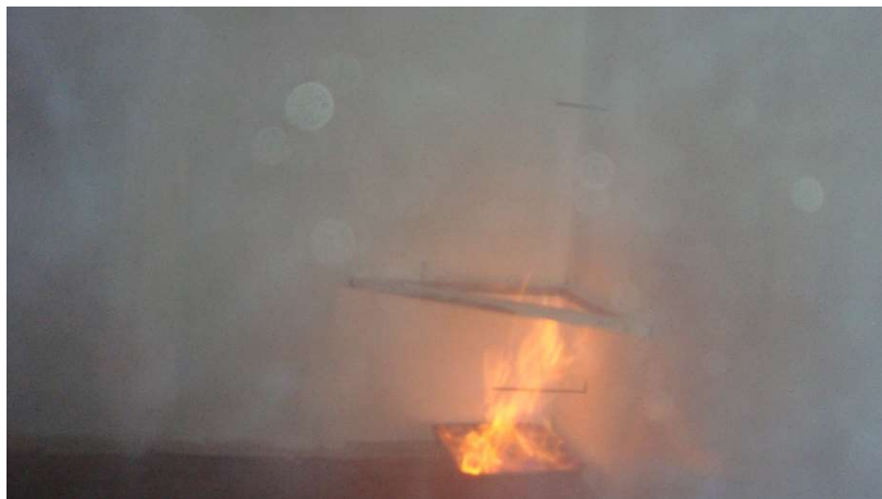
Fig. 22. Image after 30 seconds of pumping water into the enclosure at water temperature for suppression of 40 °C
