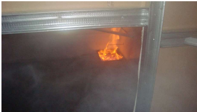
Fig. 21. Image after 30 seconds of pumping water into the enclosure at water temperature for suppression of 30 °C
