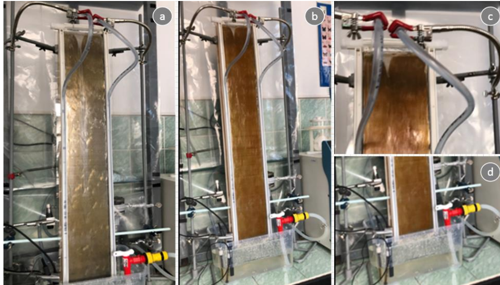
Figure 5. 5 Experimental stage after 30-60 min: a) black steel sheet surface after 30 min; b) black steel sheet surface after 60 min; c) middle area after 60 min;
