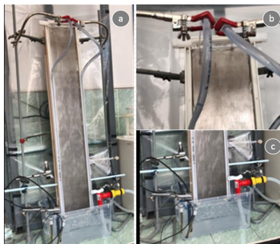
Figure. 5. 4 Initial stage at the beginning of the experiment: a)-section of black steel sheet without corrosion; b)-top of the nozzle area, initially; c)-initial supply tank.
