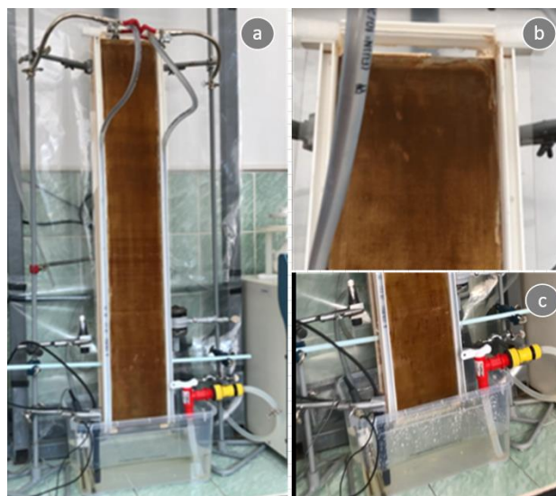
Figure 5. 7. Corrosion stage on black steel sheet surface on day III of the experimental study
