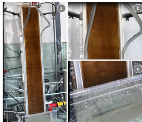
Figure 5.9 Corrosion stage on black steel sheet section on day V of the experimental study
