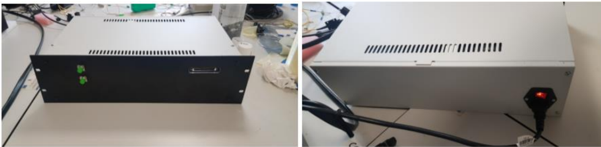
Fig. 6. 4 Final result of the box assembly for the short-range detection platform (front and back view with the cover on)
