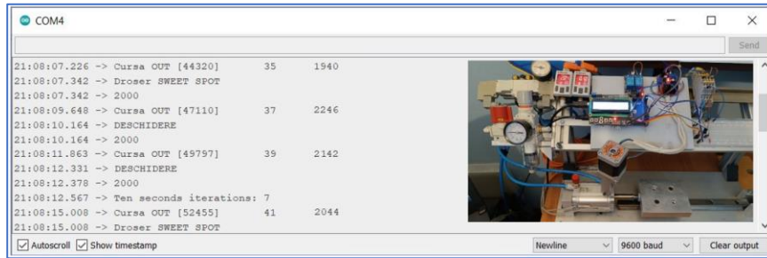
Fig. 6.21 Data acquisition at 2 bar with 0kg load for pneumatic cylinder 3
