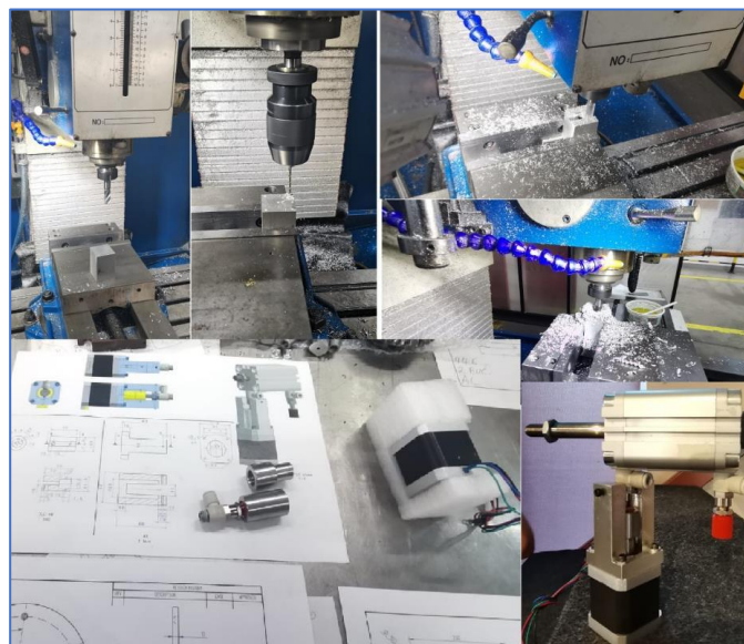
Fig. 4.8 Execution and finished product made in CATIA
