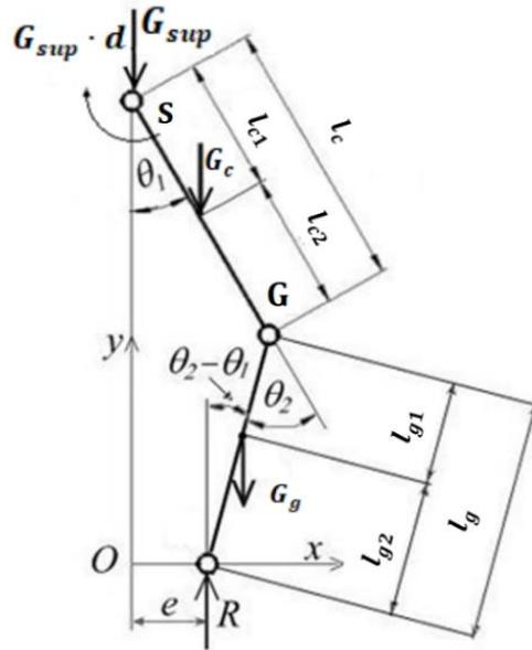
Figure 6.1. The simplified geometric model of the lower limb, consisting of the thigh and calf.
