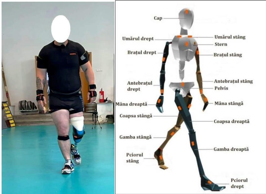
Figure 6.3. Positioning of the 17 MTw sensors on the analyzed subject.
