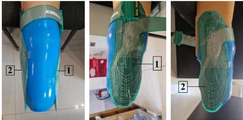
**Figure 6.20.** Placement of sensors on the residual limb: sensor 1 is fixed on the external side of the residual limb and sensor 2 on the internal side of the residual limb.
