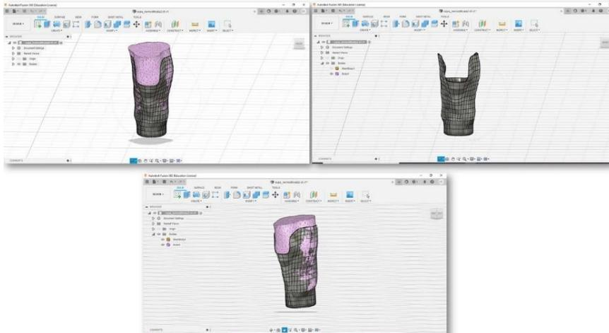
**Figure 3.3.** Visualization of the prosthetic socket on the residual limb, made in Fusion 360 software according to technical-scientific requirements.
