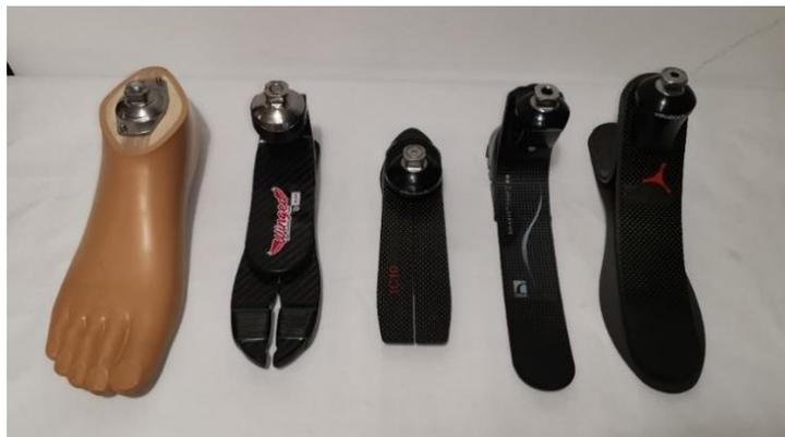
**Figure 4.1.** Prosthetic feet were tested and evaluated in this study. From left to right: SACH (Ottobock), Balance Foot J (Ossur), Winged Foot (IB-ER Prosthetic), Terion 1C10 (Ottobock) Trias 1C30 (Ottobock).
