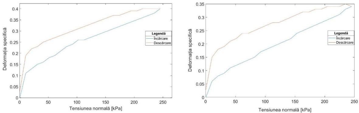
**Figure 6.19.** Deformation characteristics of commercial silicone liners a) MC97228 (Ossur) and b) SPDTHD (ALPS South Italy)
