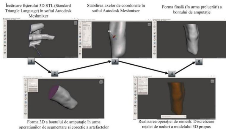
**Figure 3.1.** Processing of the STL file with the scanned amputation residual limb and the final shape (after processing with Meshmixer) of the amputation residual limb.
