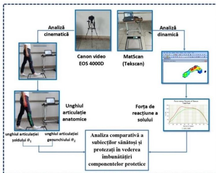
Figure 5.1. Diagram of prosthetic gait analysis with Tekscan equipment and Kinovea software for comparative analysis of normal and prosthetic human gait.
