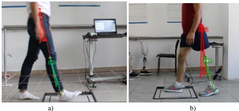
**Figure 5.2.** Positioning of landmarks on a healthy subject (a) and on a prosthetic subject (b) to measure the hip and knee angle and record the reaction force.
