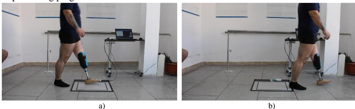
**Figure 6.7.** The beginning (a) and the end (b) of the gait cycle for the prosthetic foot, recorded with the MatScan equipment (Tekscan).
