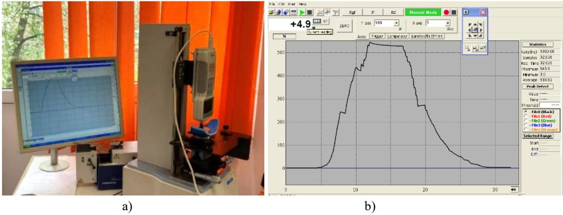
**Figure 6.17.** a) Experimental stand with samples of the three different types of prosthetic liner materials; b) force variation over time.
