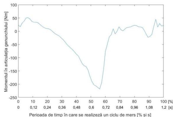
**Figure 6.9.** The variation of the actuation moment from the knee of the prosthetic leg.
