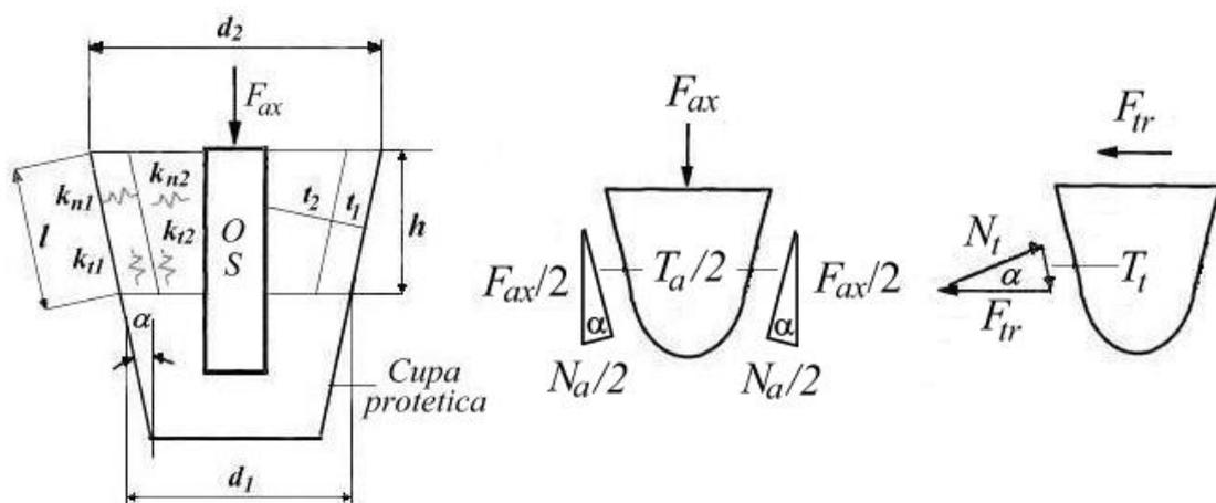
**Figure 6.15.** Simplified model of prosthetic residual limb-socket loading [49].
