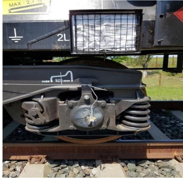
Fig.6.3.The accelerator mounted on the first axle of the first Fig.6.4.The accelerator mounted on two axles of the first
