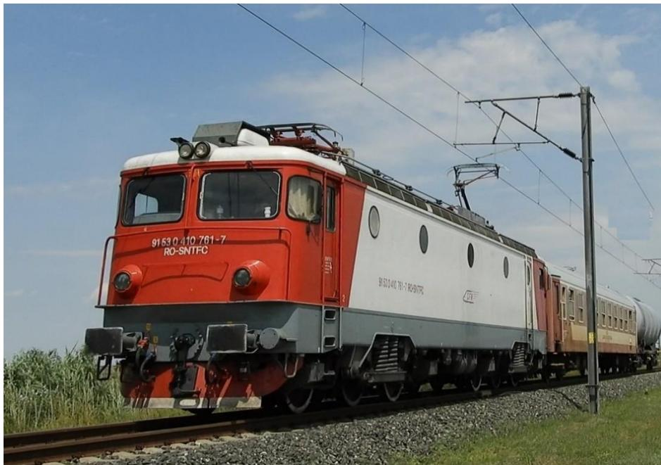
Fig.7.2. The train with which the measurements were made All 6 accelerometers are connected to the data acquisition system in the laboratory wagon.
