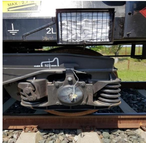
Fig.6.3. The accelerator mounted on the first axle of the first bogey
