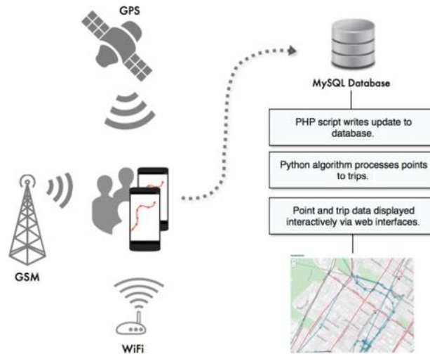
Fig. 3.8 Mobile application architecture for data processing (source: Patterson și Fitzsimmons, 2016)
