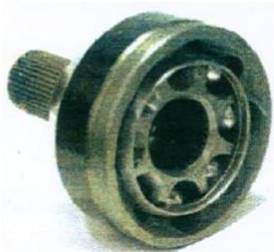
Fig. 2.7 Picture of a bowl-balls joint [G.R.18]
