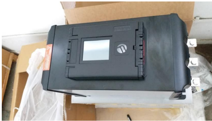
Fig. 8 – Soft starter expander Fairford SGY-305-4-01
