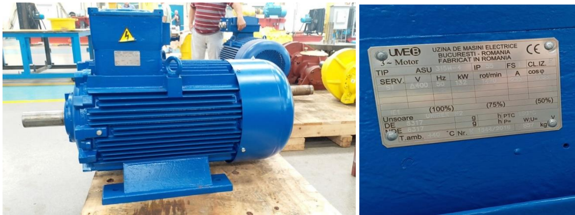
Fig. 6 – (left) The ASU 315M 132 kW electric machine (UMEB company) / (right) The label with its characteristics
