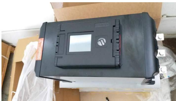
Fig. 8 – Softstarter expander Fairford SGY-305-4-01
