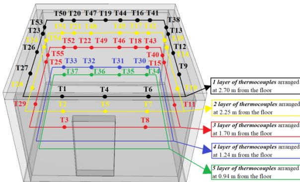
Fig. 4.7. Layered arrangement of the 55 thermocouples inside the test room
