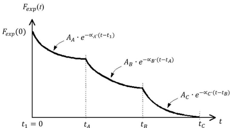
**Fig. 7.1.** Graphic representation of firefighting procedures used during an intervention in the form of the sum of exponential functions [39]
