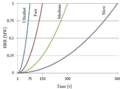
**Fig. 2.7.** Heat release rate for the fire model „t<sup>2</sup>” [18]
