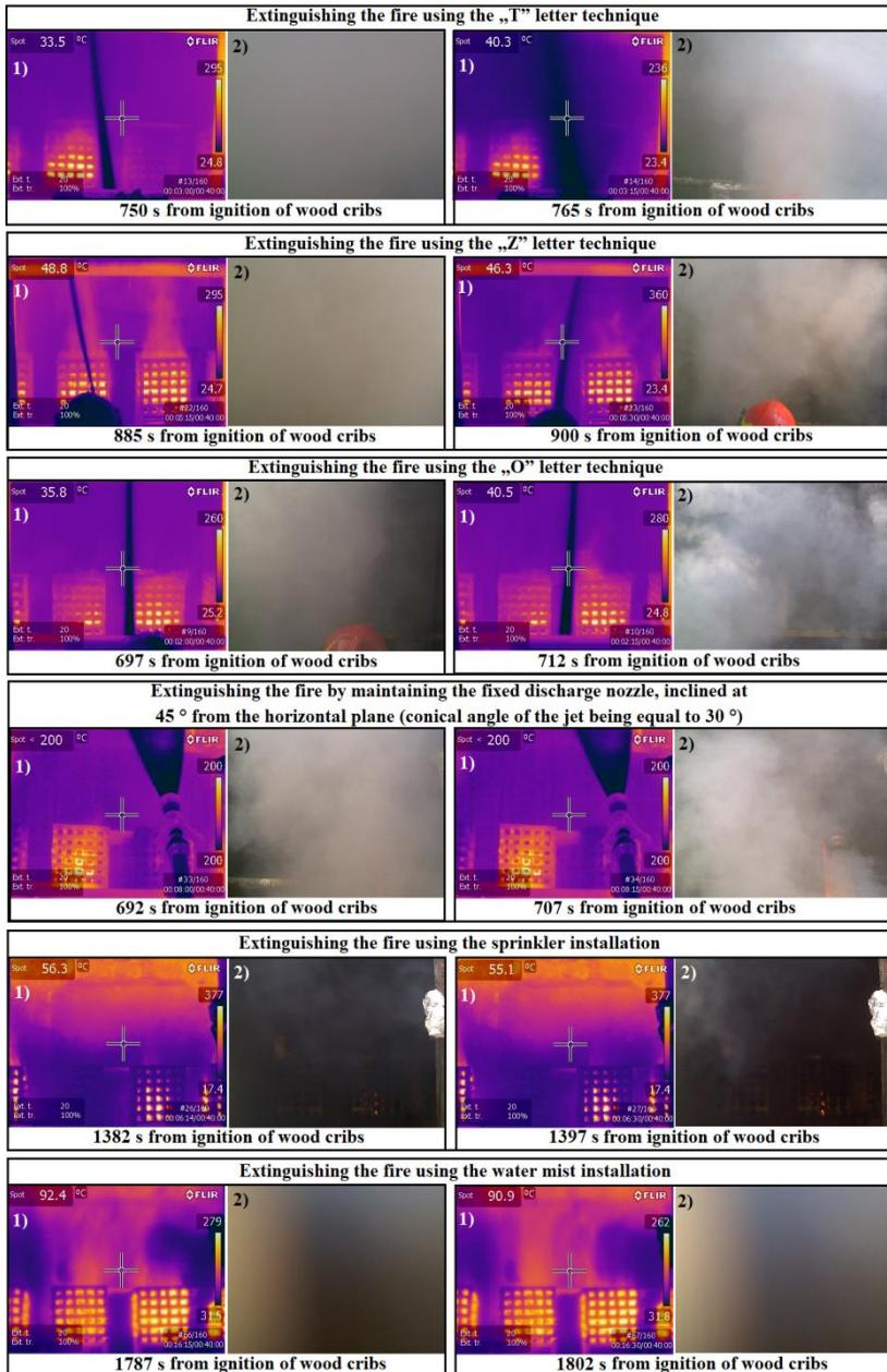
Fig. 6.10. Snapshots made at the time of temperature drop below 60 °C at a height of 1.70 m from the floor: 1) infrared image; 2) normal image.
