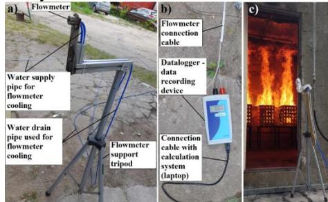
**Fig. 4.9.** The SBG01 type flow meter: a) Flowmeter; b) Datalogger; c) location mode.
