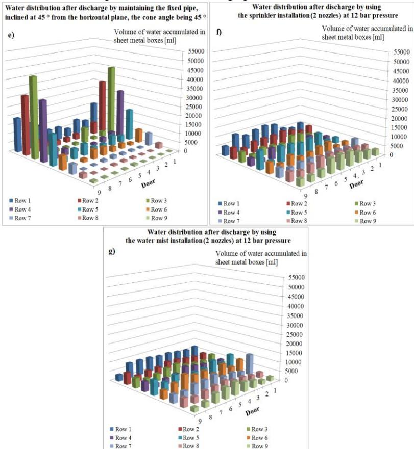
**Fig. 6.2.** Water distribution after water discharge inside the test room: e) keeping the pipe in front of the door, in a fixed position, inclined at 45° from the horizontal plane, the cone angle of the jet having a value of 45°; f) using the sprinkler installation; g) using the water mist installation.
