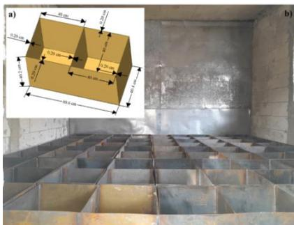
**Fig. 4.10.** Location of the 81 sheet metal boxes intended for accumulating discharged water: a) dimensions of a set of boxes; b) the location of the sheet metal boxes
