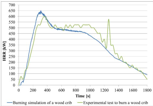
**Fig.** Error! No text of specified style in document.**8.** Comparative analysis of HRR variation over time based on the results obtained in the experimental test and simulation using the PyroSim program to burn a wood crib [11]
