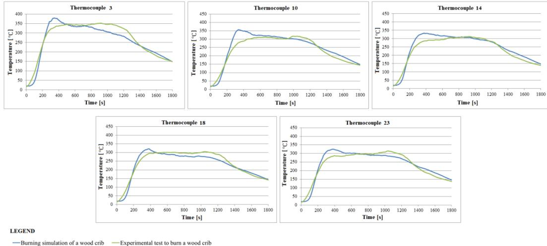
**Fig. 2.9.** Comparative analysis of the variation in temperature recorded by the thermocouples of layer 1, located at 2.80 m from the floor, based on the results obtained in the experimental test and the numerical simulation using the PyroSim program for burning a wood crib [9]
