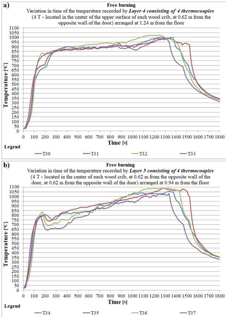
**Fig. 6.4.** Temperature values recorded by thermocouples arranged in layers, located in the stack area, relative to the floor, at: a) layer 4 – 1.24 m; b) layer 5 – 0.94 m.
