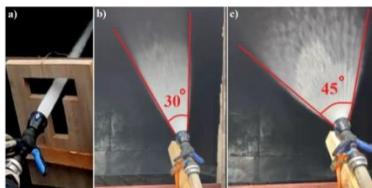
Fig. 4.4. Types of jets used in experimental tests
