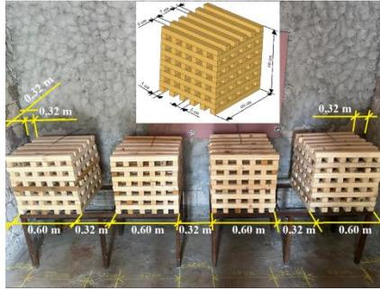
**Fig. 4.2.** Location of the 4 wood cribs that are the ignition source
