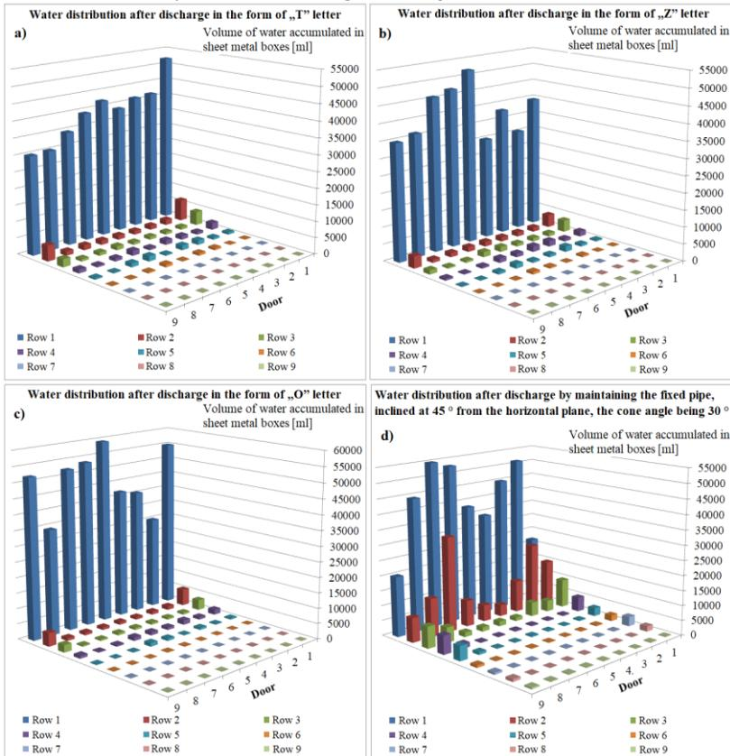
**Fig. 6.1.** Water distribution after discharge inside the test room at the door: a) using the „T” letter technique; b) using the „Z” letter technique; c) using the „O” letter technique; d) maintaining the fixed pipe, inclined at 45° from the horizontal plane, the cone angle of the jet having the value of 30°.
