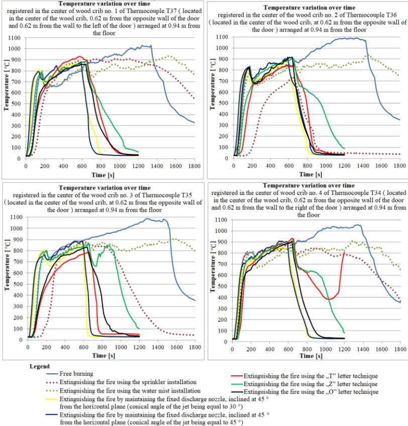
**Fig. 6.9.** Variation in time of the temperature recorded in the center of the wood crib by thermocouples of the layer 5
