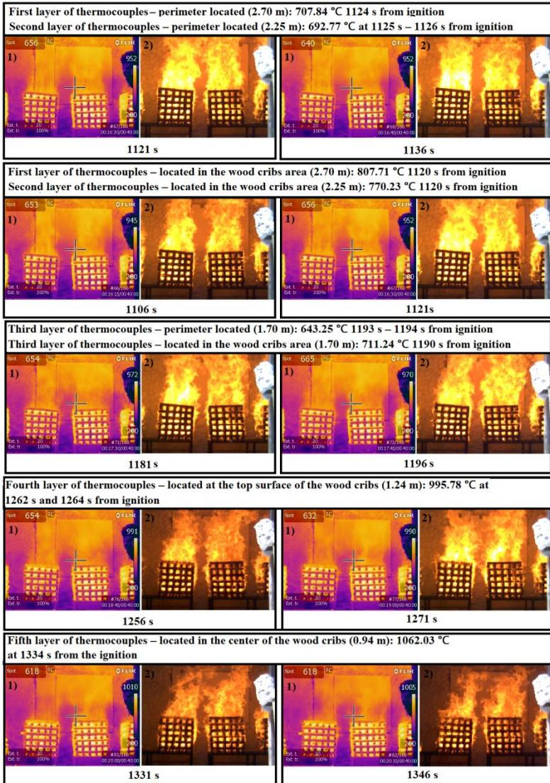
**Fig. 6.5.** Snapshots made when reaching the maximum temperature average values recorded by thermocouples on each layer: 1) infrared image; 2) normal image.
