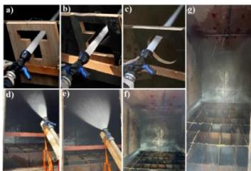
**Fig. 4.11.** Water discharge using: a) letter technique „T”; b) letter technique „Z”; c) letter technique „O”; d) discharge nozzle inclined at 45°, cone angle being equal to 30°; e) discharge nozzle inclined at 45°, cone angle being equal to 45°; f) sprinkler installation; g) water mist installation.
