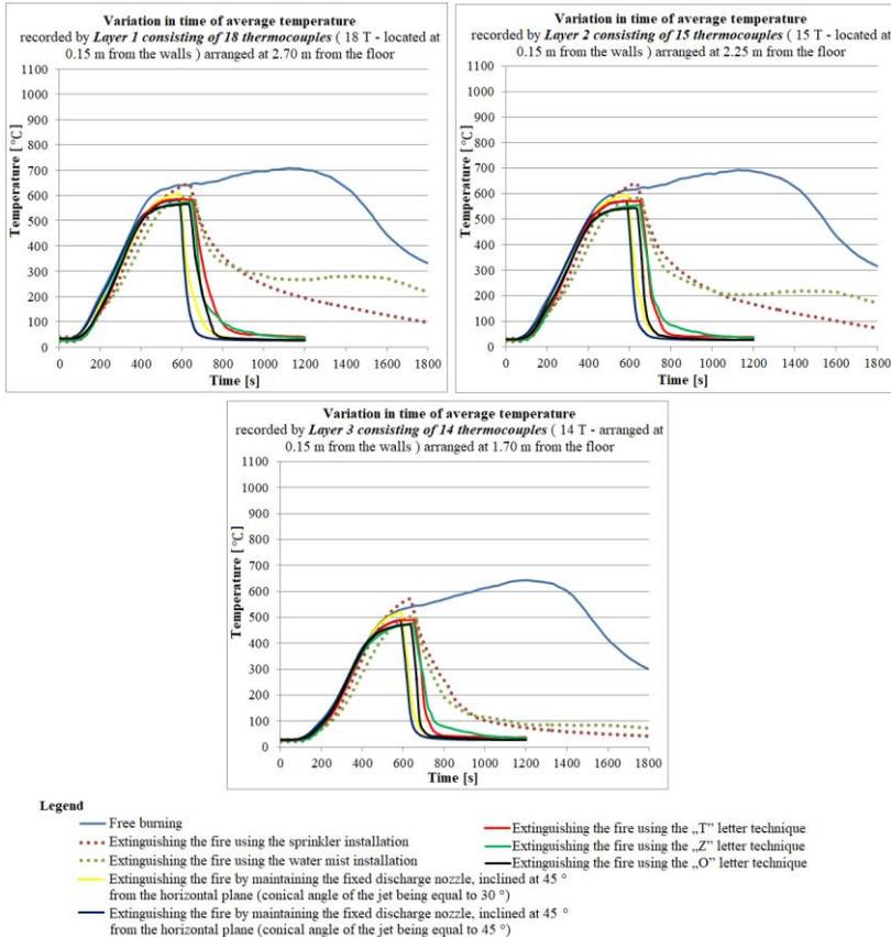
**Fig. 6.7.** Variation in time of the average temperature recorded in the test room of the thermocouples of layers 1, 2 and 3
