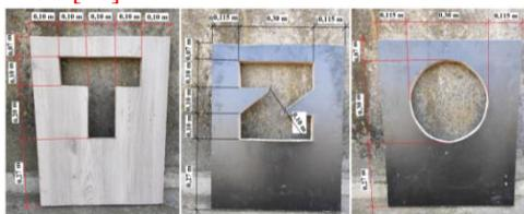
Fig. 4.6. The „T”, „Z”, „O” models by which water is discharged
