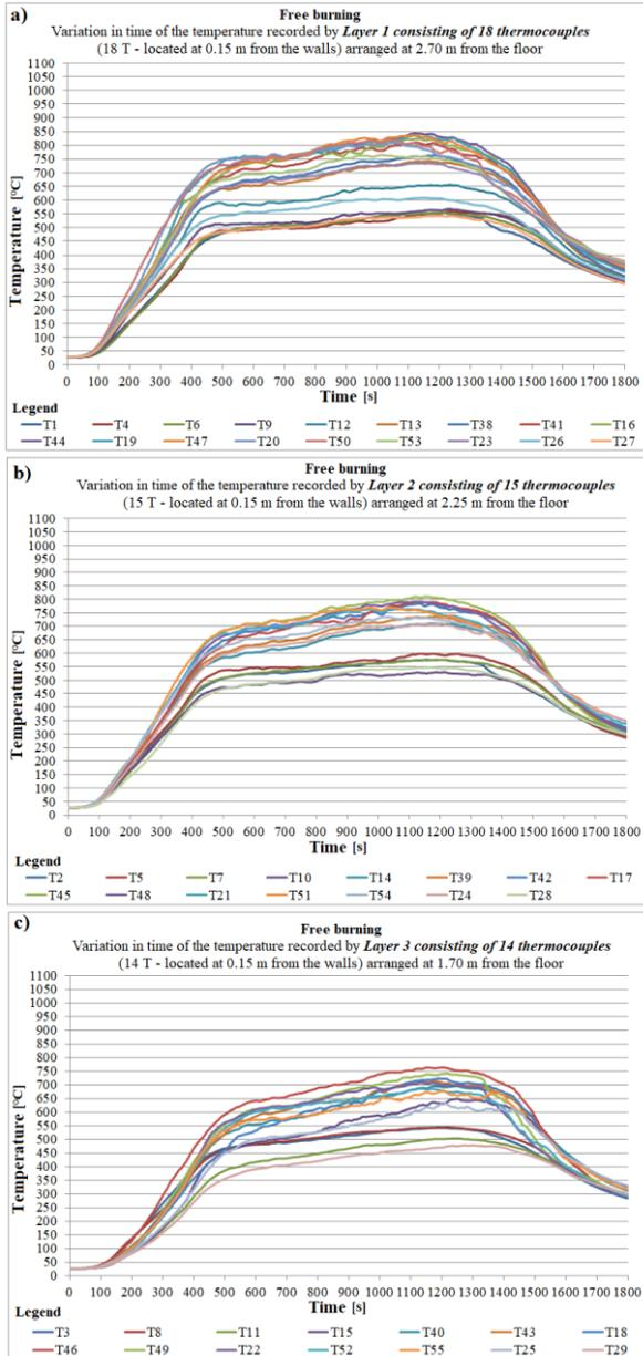
**Fig. 6.3.** Temperature values recorded by thermocouples arranged in layers, located perimetrically, inside the test room, compared to the floor at: a) layer 1 - 2.70 m; b) layer 2 – 2.25 m; c) layer 3 - 1.70 m.
