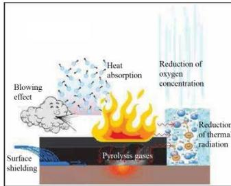
Fig. 2.2. Fire extinguishing water mechanisms using nozzles [19]
