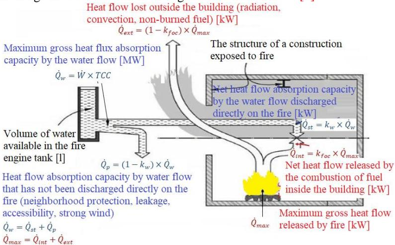
**Fig. 2.3.** Energy balance on the capacity of the water flow absorption of the heat flow and the capacity of the fire to produce the heat flow [2]
