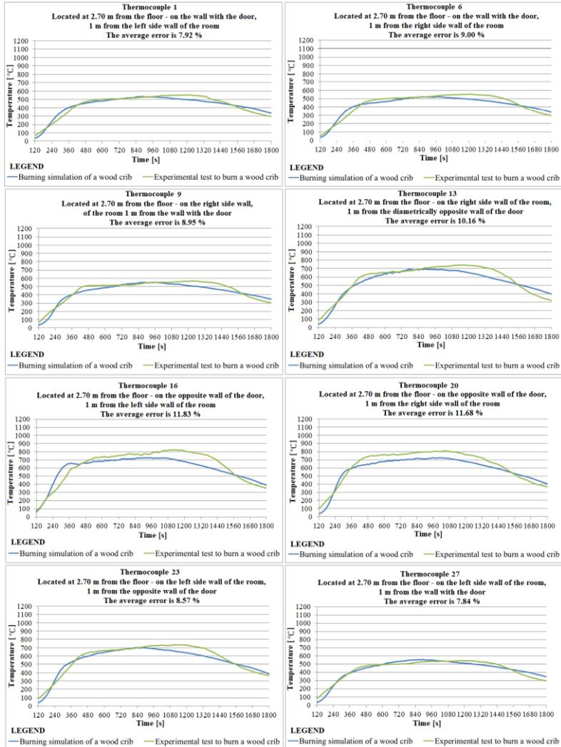
Fig. 6.6. Time variation of the temperature obtained from the experimental free combustion test of four wood cribs compared to the simulation using the PyroSim program
