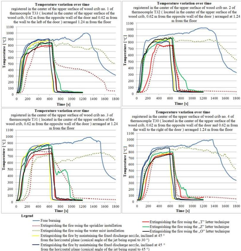
**Fig. 6.8.** Time variation of the temperature recorded in the middle of the upper surface of the wood crib by thermocouples of the layer 4
