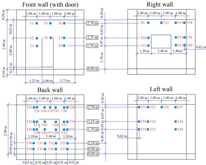
**Fig. 4.8.** Location of thermocouples – view from outside the test room
