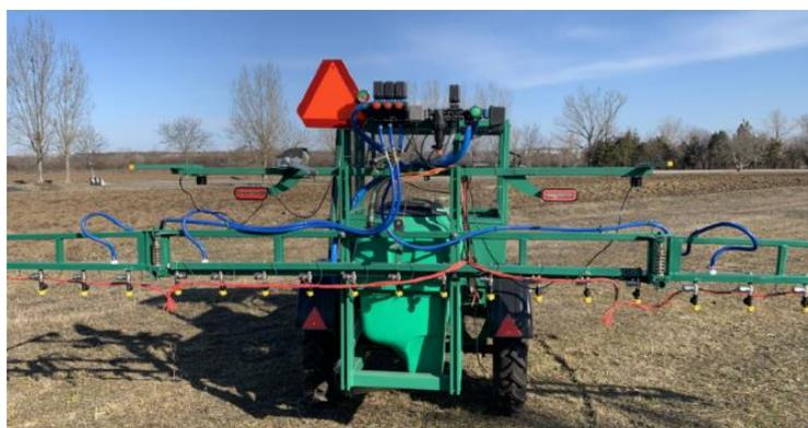
Figure 5.11 The electric vehicle intended for spraying work in field tests
