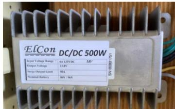
Figure 4.15 500W EICon DC/DC converter
