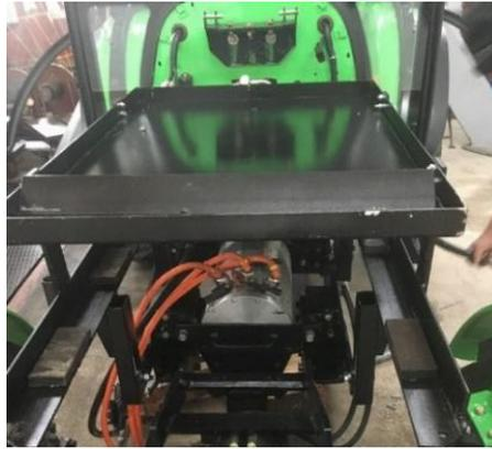
Figure 5.6 Battery holder and electronic control system completed
