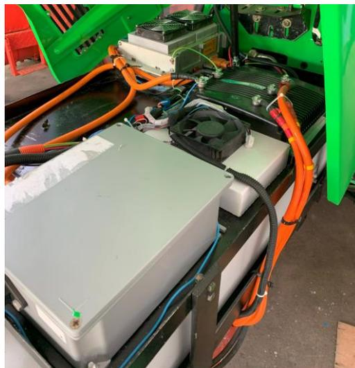
Figure 5.7 Detail from the installation of the electronic equipment on the electric tractor
