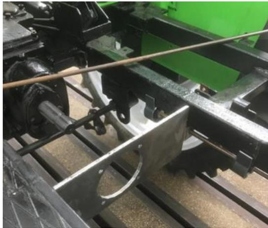
Figure 5.1 The mounting system of the electric motor to the chassis of the electric vegetable tractor
