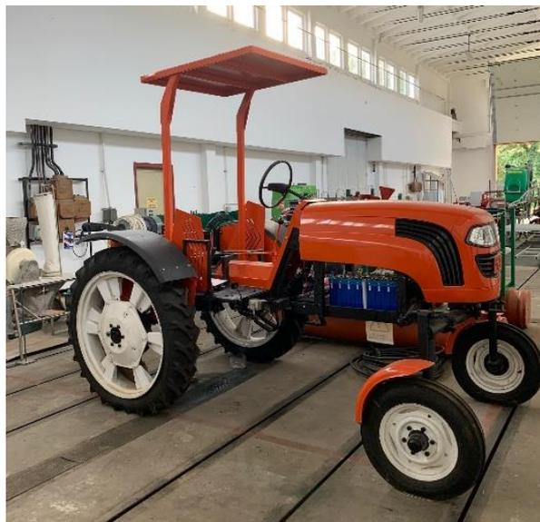
Figure 5.10 Electric transport tractor
