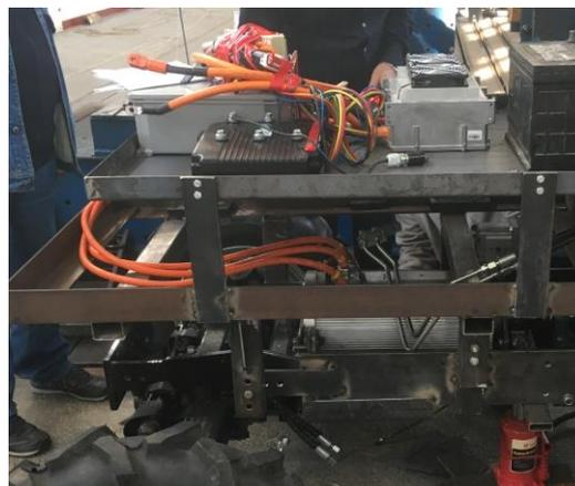
*Figure 5.5 Details of the battery and electronic engine control system mounting system*
