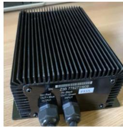
Figure 4.14 DC/DC Converter
