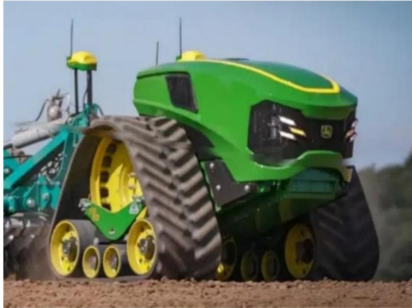
Figure 2.2 John Deere autonomous electric tractor [9]
