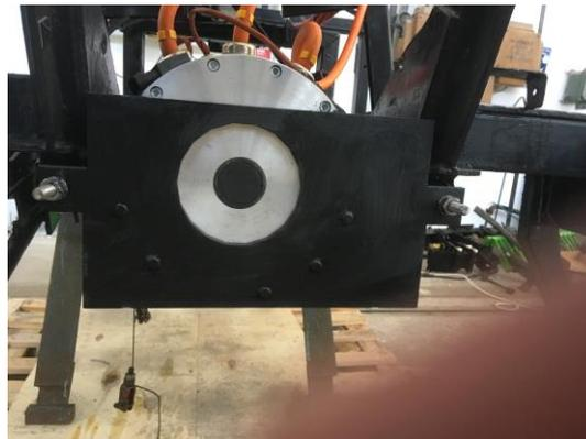
Figure 5.2 Mounting the engine on the chassis
