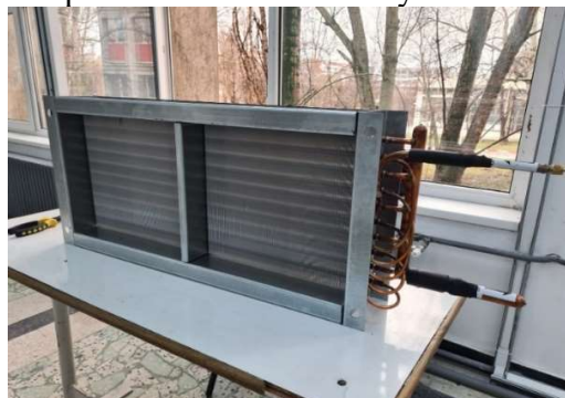
Fig. 4.1 The evaporator in the air handling unit
