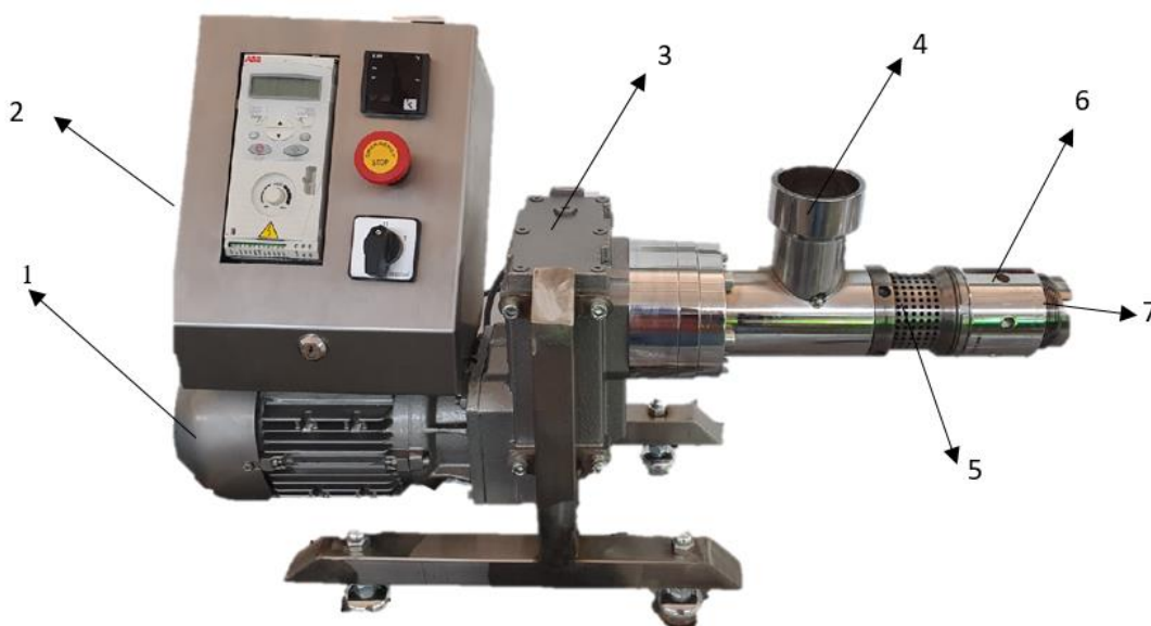
Fig.6. 32 Screw press NF 80: 1- motor; 2- control panel; 3- reducer; 4- press feeding area; 5- oil discharge area; 6- the pressing head; 7- the discharge nozzle of the meal.
