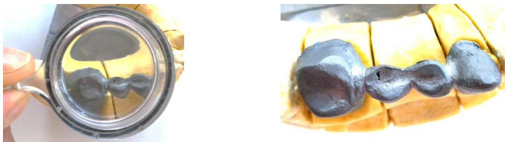
Figure 4.12. Detecting the presence of pores
