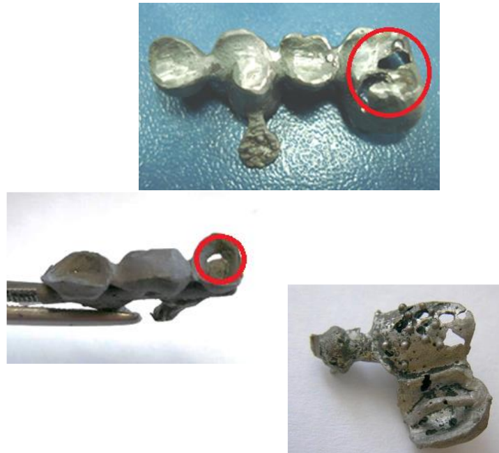
Figure 4.13. Partial gaps in cast metal frames
