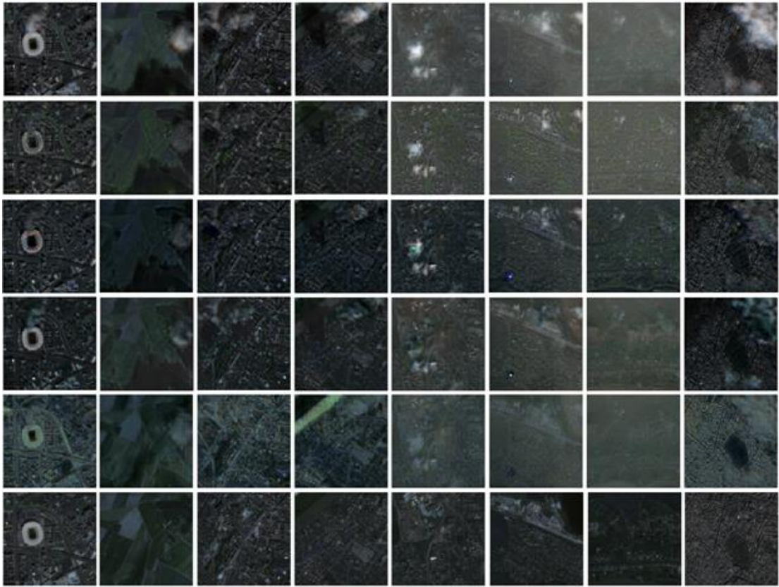
Figure 4.8: Qualitative results, Row I: cloudy test samples, Row II: results of RGB, Row III: results of RGB+IR, Row IV: results of full bands, Row V: results of Hybrid GAN-SAD, Row VI: ground truth.
