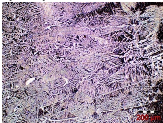
Fig. 4.14. Dendritic microstructure of HT alloy 3. Optical microscopy. LAMET laboratory.
