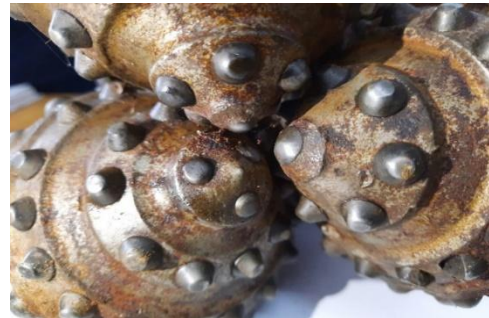
Fig. 2.9 . Image of the core area of a three-roller drill bit with advanced tungsten carbide insert wear [11].
