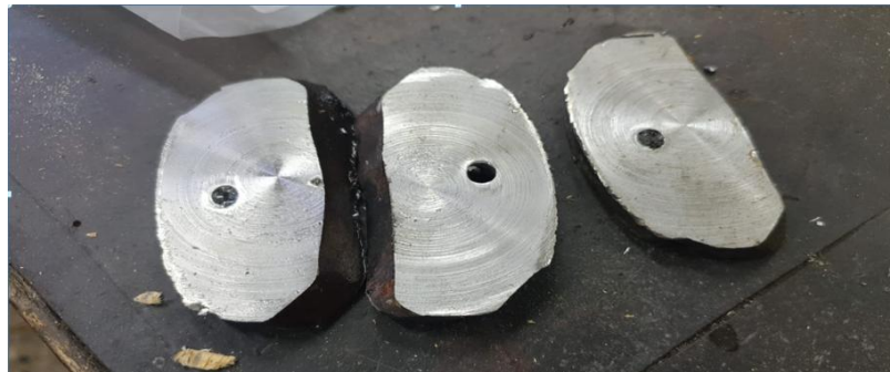
Fig. 5.40. Samples taken from the drilling bit to be loaded by welding.
