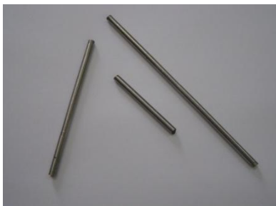
Fig. 4.6. S2 HT 3 alloy rods resulted from mechanical processing by turning.
