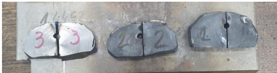
Fig. 5.41. Cross-sections through the samples loaded by welding with the HEA 6 alloy.
