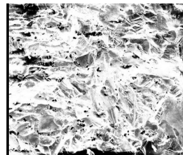
Fig. 2.16 . Equiaxial grainning in a high-entropy AlCrFeMnNi ingot [16].
