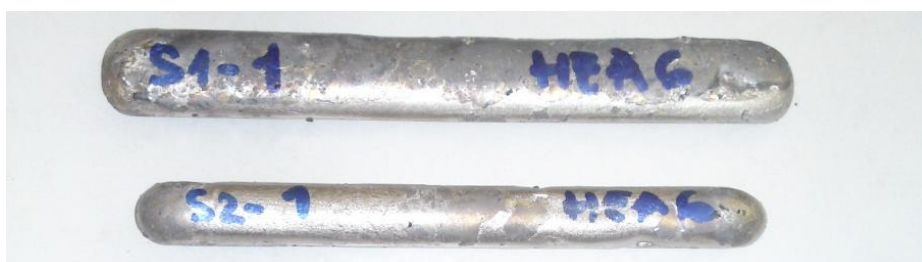
Fig. 4.7. Appearance of mini-ingots obtained from AlCoCrFeNi alloys.
