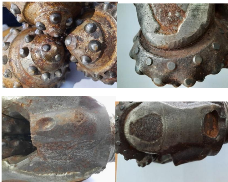
Fig. 5.1. Visual examination of the 3-cone drill bit and highlighting the level of wear of the ceramic elements and the areas with gripping welds of the cones.
