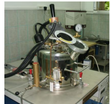
Fig. 4.1. The RAV – MRF ABJ 900 facility with which the experimental high entropy alloys were obtained. ERAMET Laboratory, UPB.
