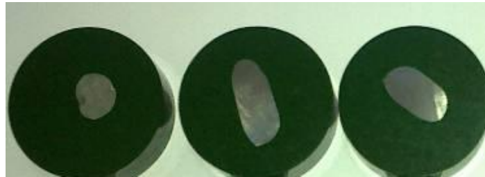
Fig. 4.10. Appearance of AlCrFeMnNi alloy samples after embedding in resin.
