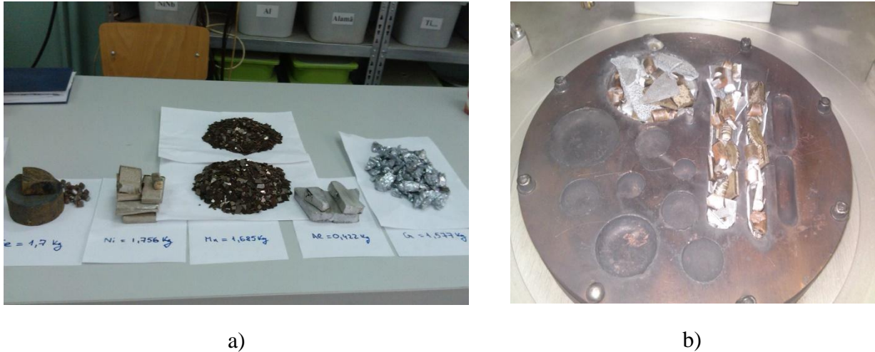
Fig. 4.2. Preparation of raw materials (a) and distribution of metal charge elements on the melting plate in the RAV facility (b).
