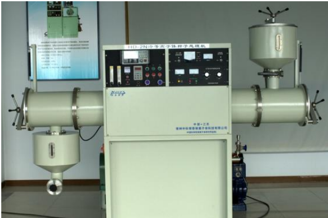
Fig.15. Echipament de tratat semințe prin utilizarea plasmei reci HD-2N Cold Plasma Seed Processor (Changzhou Zhongke Changtai Plasma Technology Co., Ltd)
