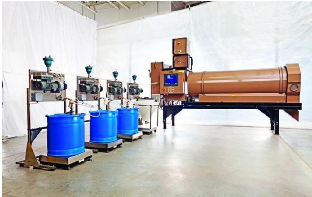
Fig.5. Echipament industrial de tratat semințe, On Demand, Bayer, [12]
