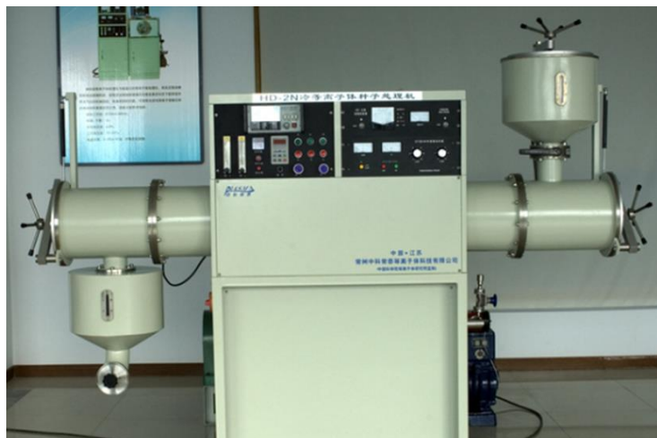
Fig.15. HD-2N Cold Plasma Seed Processor (Changzhou Zhongke Changtai Plasma Technology Co., Ltd)
