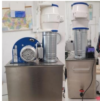
Fig. 17 Realization of the assembly of the industrial air filtration system based on the phenomenon of ultrasonic cavitation: a - frontal view; b - side view
