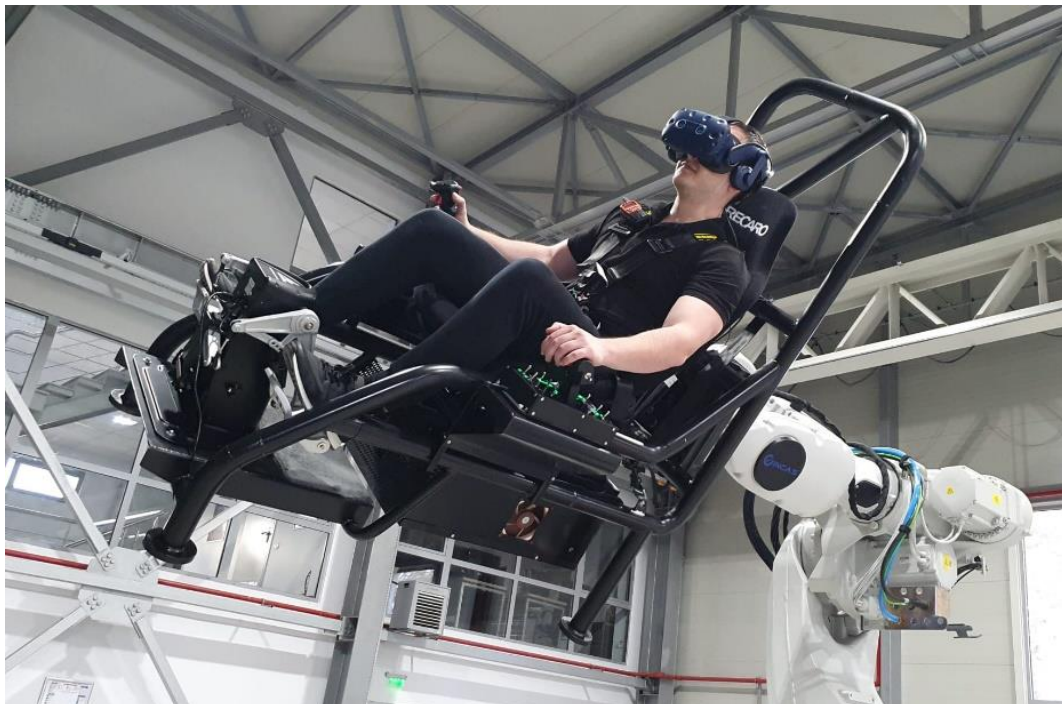
Figure 3.1 Dynamic simulation system for pilot-in-the-loop applications, Credits: INCAS
