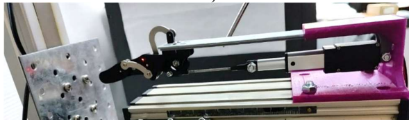
Fig. 8.38. Actual locations where the system was hit to start measuring vibration
