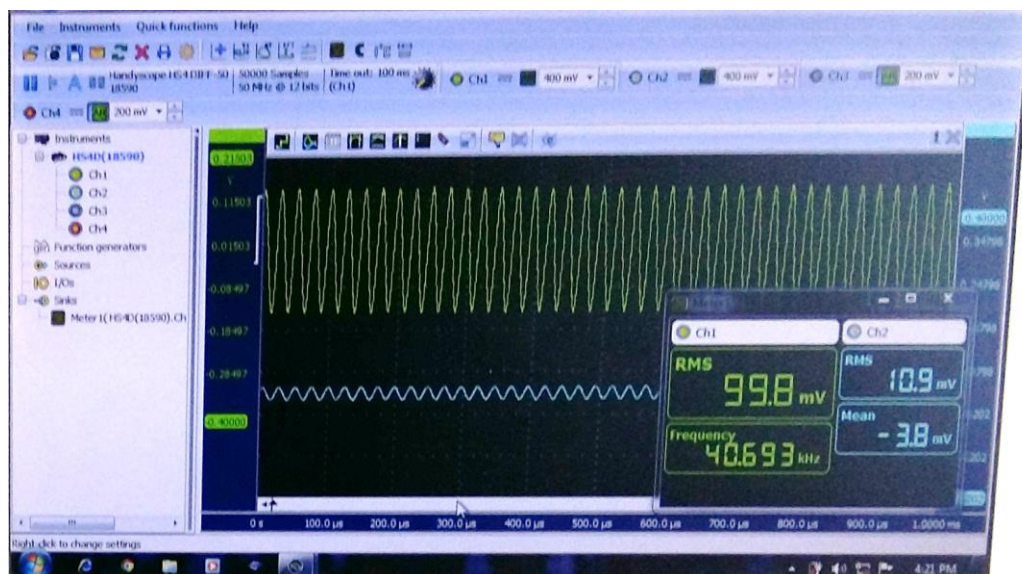
Figure 9.2 Detail of the digital oscilloscope screen with the determination of the resonance frequency at 40693 kHz
