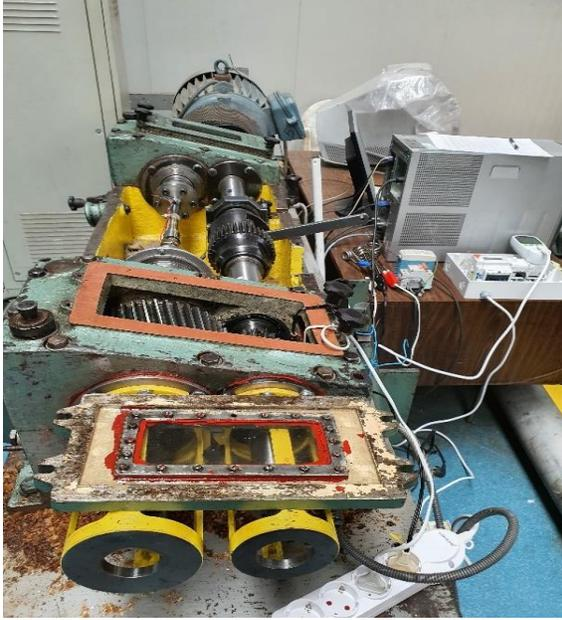
Fig. 5.11. The testing rig for gears and lubricants equipped with electric resistors, a socket with a digital energy meter, and a voltage variator
