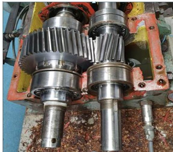
Fig. 2.43. Lower half housing, with mounted gearing, made at Cugir Mechanical Plant
