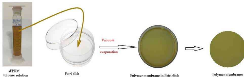
**Figure 2.** Schematic presentation of obtaining the polymer membrane (sEPDM) or of the composite membrane (Chi/sEPDM)
