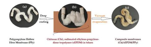
Figure 1. Schematic presentation of getting the composite membrane (Chi/sEPDM/Ppy)
