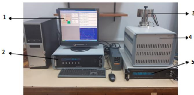
Fig. 6.1. Dielectric Spectrometer 1 – PC; 2 – Central unit; 3– Measuring cell; 4 – NovoTherm temperature control system; 5 – Command unit;
