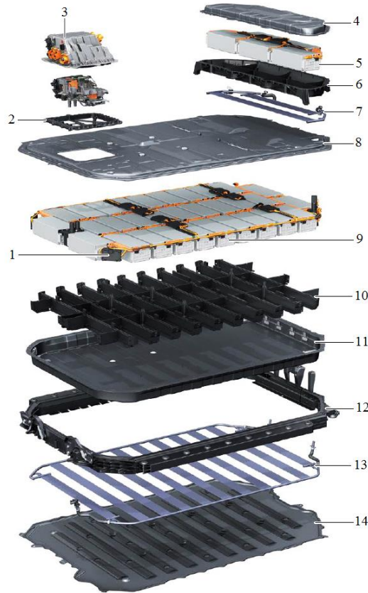
Figura 2.24. Construction of a lithium-ion battery, [50]:
