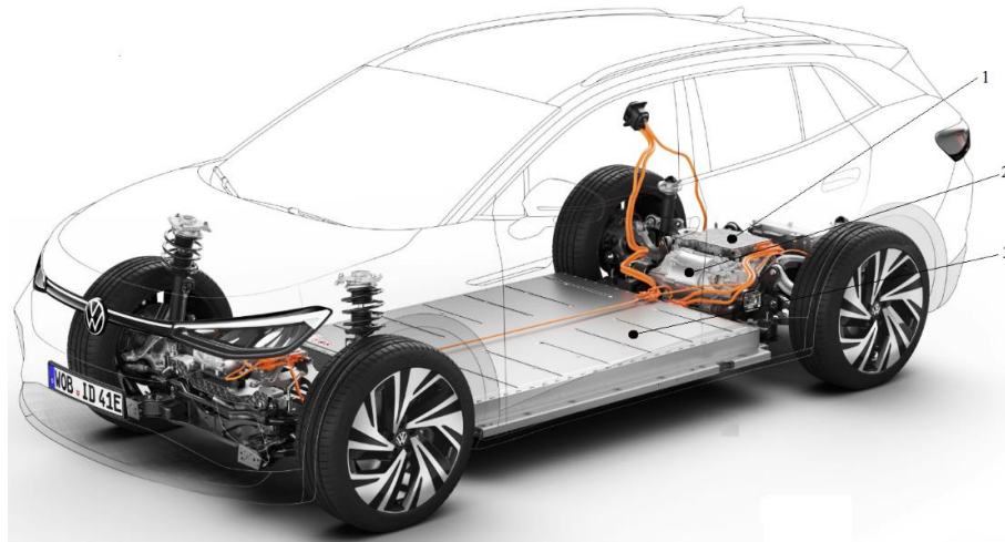
Figura 2.5. Architecture of the VW ID.4 vehicle, [13]: 1 – Speed variator; 2 – Electric motor; 3 – Lithium-ion battery.
