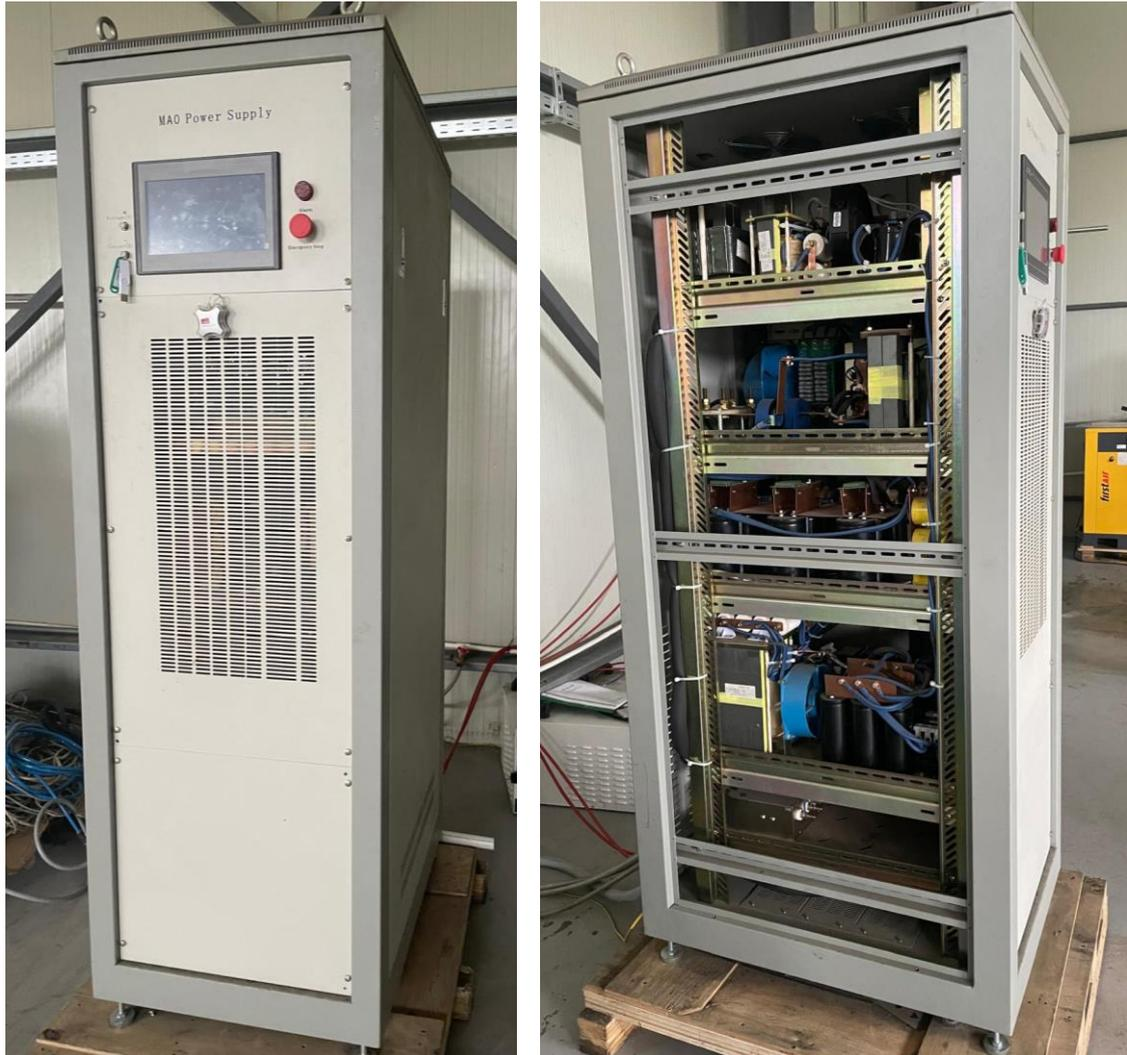
*Figura 3.4. Overview images - Plasma Technology power supply for industrial PEO plant*
