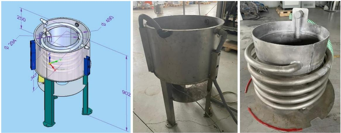
Figura 3.5. CAD design and construction - bowl with electrolyte cooling and recirculation system
