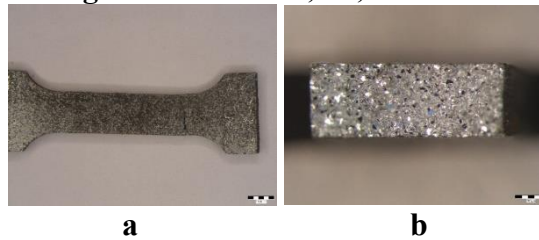
Fig. 3.14-Macroscopic appearance of the ZnMg tensile specimens after annealing at 300°C/ 5h: a- longitudinal section, x8; b- cross-section, x40
