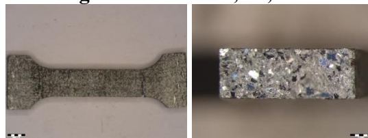
Fig. 3.20-Macroscopic appearance of the ZnMgFe tensile specimens after annealing at 300°C/ 10h: a- longitudinal section, x8; b- cross-section, x40
