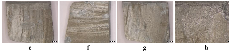
Fig. 4.5. - Macrostructural aspects of ZnMg alloy surfaces degraded in SBF, after different immersion periods, without corrosion products: a- before testing; b- after 3 days; c- after 7 days; d- after 14 days; e- after 21 days; f- after 28 days; g- after 35 days; h- detail of the image g
