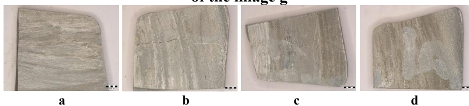
Fig.4.4. - Macrostructural aspects of zinc surfaces degraded in SBF, after different immersion periods, without corrosion products: a- before testing; b- after 3 days; c- after 7 days; d- after 14 days; e- after 21 days; f- after 28 days; g- after 35 days; h- detail of the image g
