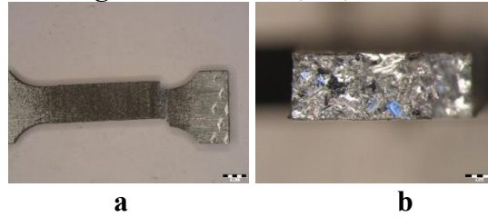
Fig. 3.12 - Macroscopic appearance of the zinc tensile specimens, after annealing at 400°C/ 10h: a- longitudinal section, x8; b- cross-section, x40
