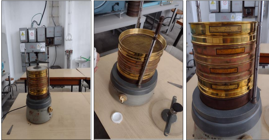
Fig. 5. 2. The image of the vibration screening device with 4 standardized sieves
