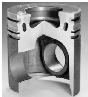
Figure 2.12. Short fibre reinforced aluminium matrix composite piston for diesel engines [12].
